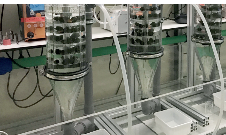
Flow-through system to determine the bioaccumulation potential of mussels. Photo: Fraunhofer IME
